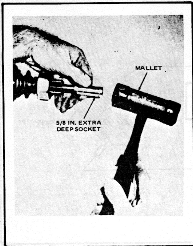
Figure 6-13. Removing Retainer from Snap Ring
